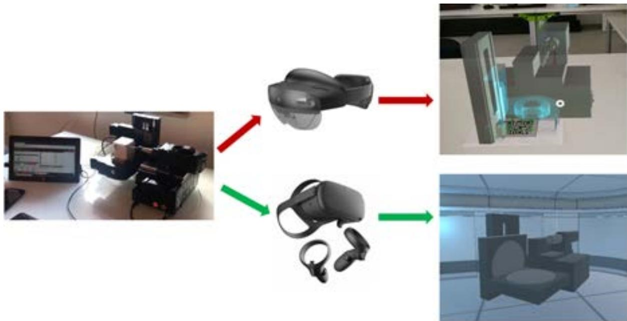
**Figure 2:** *Training on the same content (milling machine) using different technologies (VR and MR) because of different types of learners*
